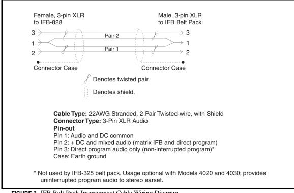
FIGURE 2. IFB Belt Pack Interconnect Cable Wiring Diagram
